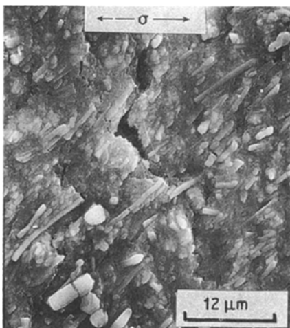
Figure 13 Crack propagating path in 45° off-axis angle specimen.
